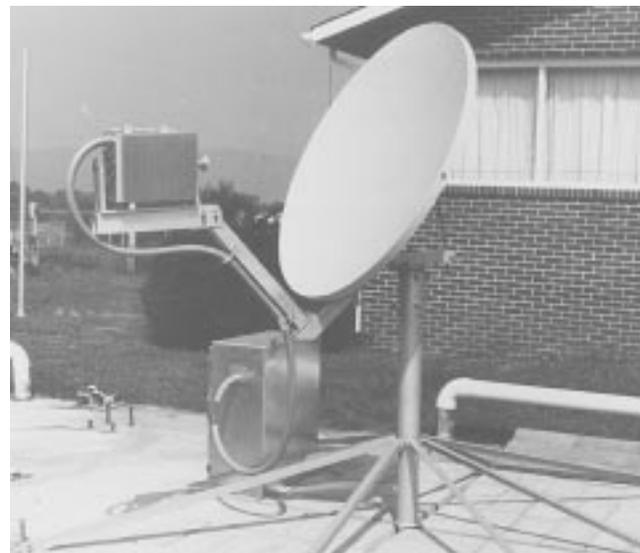
Fig. 5. ACTS 1.2-m receive-only propagation terminal.
