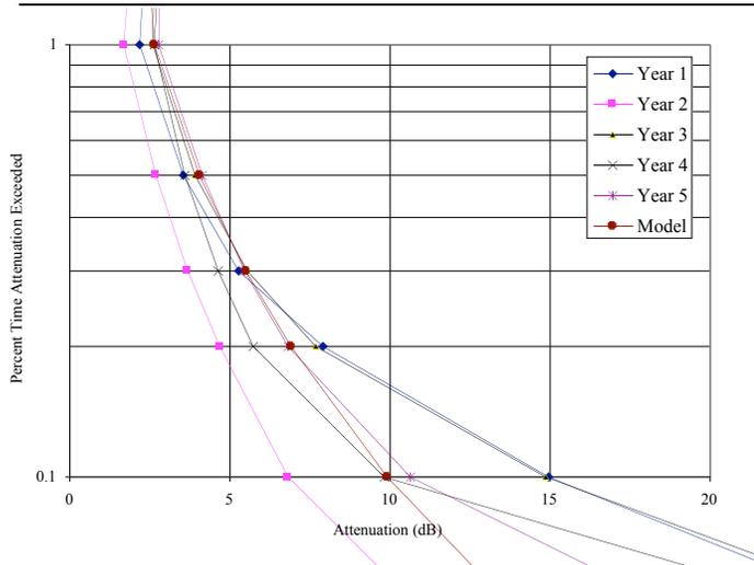
Figure 3. Rain attenuation distribution at 20.2 GHz; Reston, VA; Elevation angle is 39°
