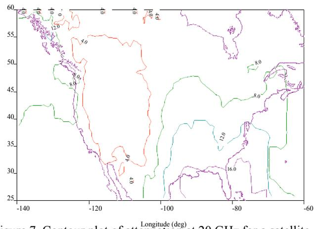
Figure 7. Contour plot of attenuation at 20 GHz for a satellite located at 100°W.
