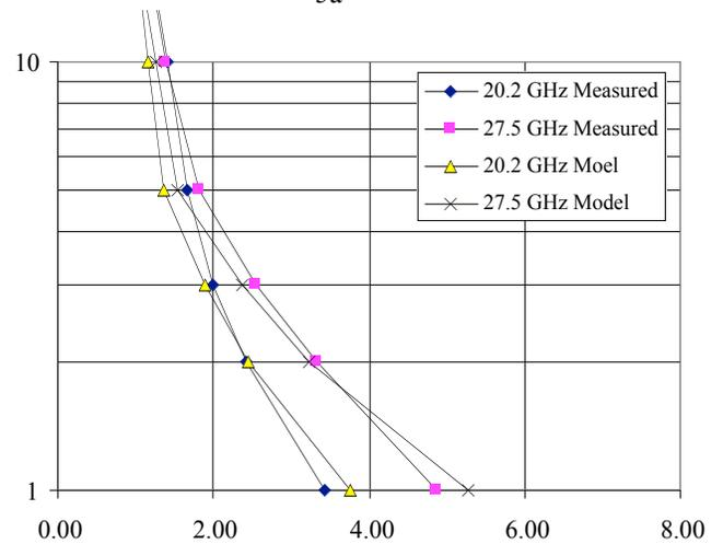
Figure 6. Attenuation distributions at 20.2 and 27.5 GHz; Clarksburg, MD; Elevation angle is 39°
