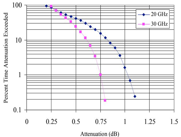
Figure 1 Gaseous absorption distributions at 20 and 30 GHz; Washington, DC; Elevation angle is 40°
