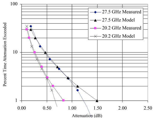
Figure 2 Cloud attenuation distributions at 20.2 and 27.5 GHz; Clarksburg, MD; Elevation angle is 39°
