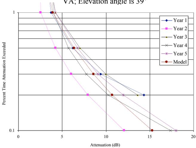
Figure 4. Rain attenuation distributions at 27.5 GHz; Reston, VA; Elevation angle is 39°
