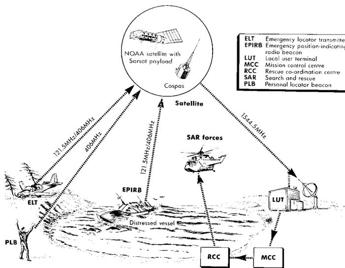
Figure 2: Basic Concept of the Cospas-Sarsat System
