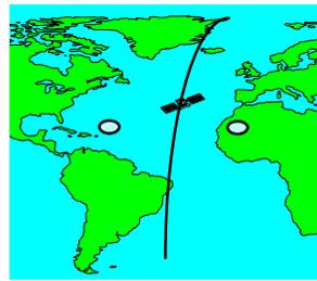
satellite pass another pair of positions would be produced, but only one of those would overlap with one from the previous pass, thus establishing which is the true position of the beacon.
