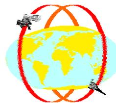
The basic Cospas-Sarsat System [1] utilizes a constellation of four low-Earth-orbit (LEO) satellites in near-polar orbit, as depicted in Figure 1. With this type of orbit, a single satellite eventually scans the entire globe.
